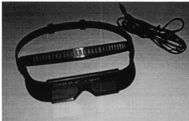
Fig.15. Prototype of stereo glasses with ergonomic headband
